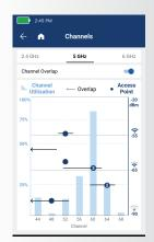
Channel test shows key information for understanding the Wi-Fi environment: number of AP's seen on and overlapping each channel and their signal strength, plus total channel utilization. Touching a channel provides details on APs on or interfering with that channel.
