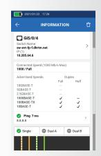
Switch port test shows switch name and IP address, connected port, and VLAN along with advertised speed and duplex settings. If a ping test is configured, the target address and average response time are shown. Scrolling down displays Power over Ethernet results.
